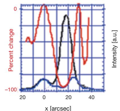
Imaged binary star system Cor Caroli through the optical vortex coronagraph with and without the vortex lens in place. The bright primary star is suppressed, whereas the weaker secondary star is unaffected. The plotted intensity curves (black, blue lines) show a peak suppression of 97 percent (red line).
