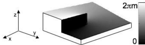
FIG. 1 A three dimensional plot of an optical vortex mask of topological charge m . The thickness of the mask (the z dimension) increases in the azimuthal direction forming a spiral shape on the upper surface of the mask. The thickness of the mask is represented by the phase shift through the mask in radians.
